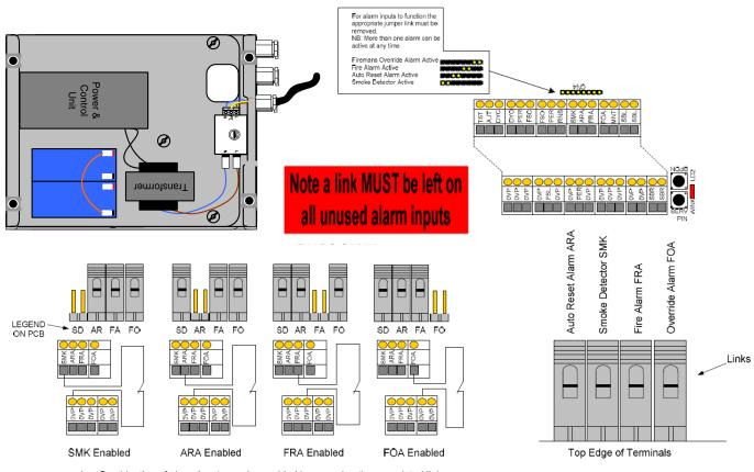
Any Combination of alarm inputs can be enabled by removing the associated links Note: Store the links by turning through 90 degrees and fitting them on to either pin
