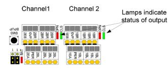
Output mode - timed off, reversing polarity Actuator Full Stroke Period (natural ventilation) – 180 seconds Alarm Full Stroke Period (Smoke Vent) - 180 seconds Over current response >8A for 2 seconds
