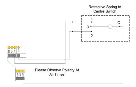
Connecting terminals DYO and DYC to 0VP will open and close the vent in natural ventilation mode. The default mode requires a spring centre 3 position switch having 2 normally open contacts. The actuator will only move whilst the input demand is in force and the total movement time in the requested direction is less than 18 seconds (default). Releasing the switch will stop the movement.
