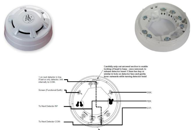
Test using Canned Smoke or other approved smoke generating method. No other method is acceptable.
