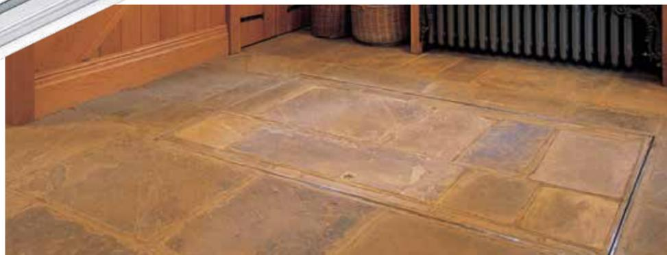
Aluminium spring-balanced floor access covers for light pedestrian traffic
