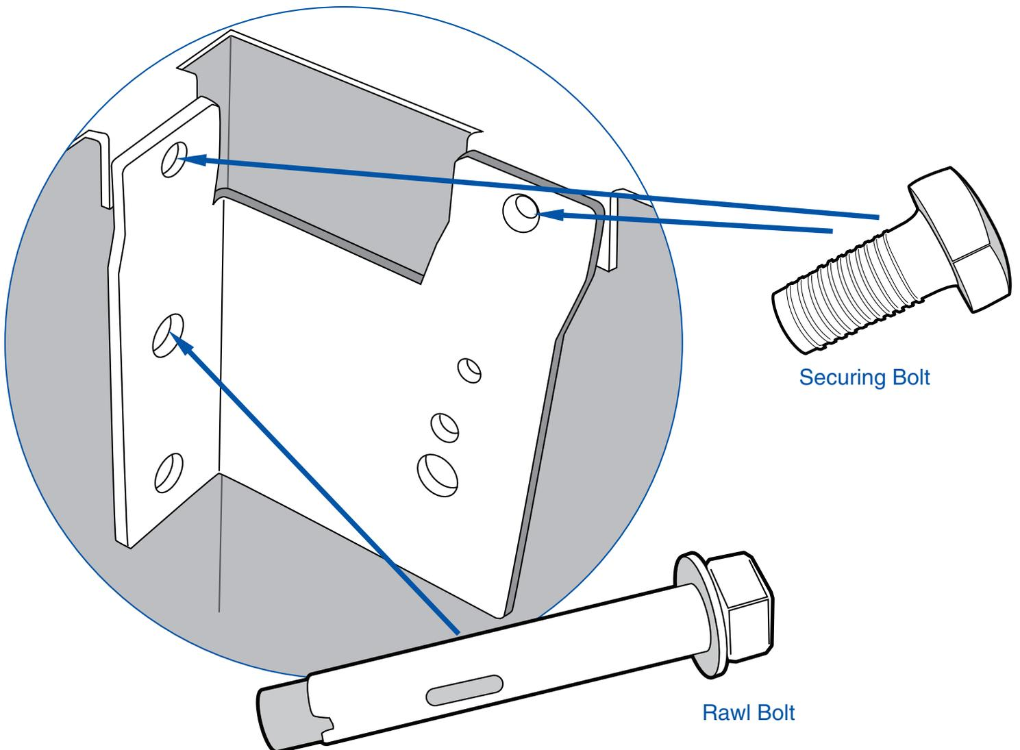
Drill holes in pit walls. Affix bracket against wall with **Rawl Bolt** and tighten **Securing Bolts**.
