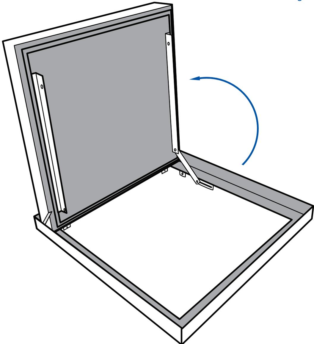
Remove the two **Hinge Bolts**,
