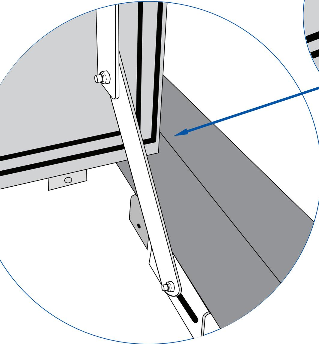
Close cover placing spacers between the cover and outer frame prior to filling and tiling. Fill cover and tile surrounding area, ensuring that the infill has the equivalent strength of 40MPa concrete when fully cured. Fix **Lifting Eyes** to cover, using bolts supplied. Open cover with **Lifting Bar**.
