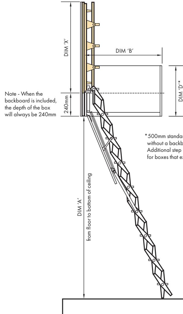
\* 500mm standard depth of a box without a backboard. Additional step is available if required for boxes that exceed 500mm
