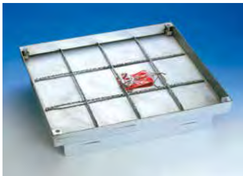
BVS-400 Galvanised Steel BVES-400 Stainless Steel Pan Depth: 50mm Load Capacity: 400kN Test Load EN 124
