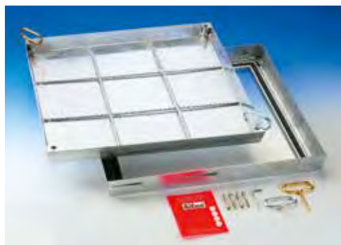
BV Galvanised Steel BVE Stainless Steel Pan Depth: 50mm Load Capacity: 125kN Test Load EN 124
