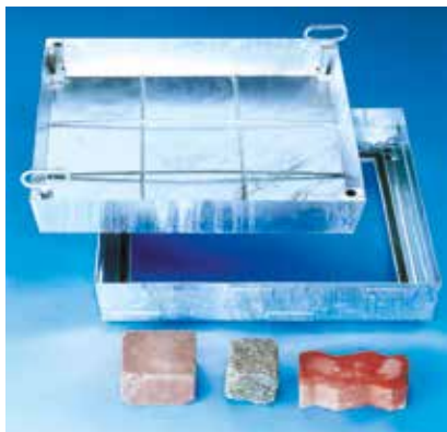
BVH-Maxi Galvanised Steel BVEH-Maxi Stainless Steel Pan Depth: 102mm Load Capacity: 125kN Test Load EN 124*
