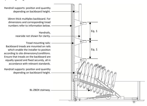
BL-ZBOX backboard 1: Up to 1000mm high by up to 1200mm wide, 18mm thick white coated multiplex board, fitted with 2-3 additional treads and grab rails.
