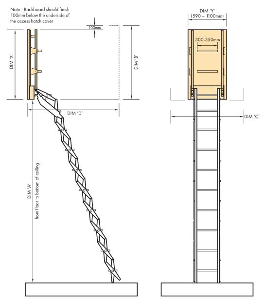
When the BL-Z is ordered with a Backboard, the BL-Z will be delivered fitted to the backboard.
